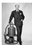
1956 Creation of the C-pump: the first-ever submersible wastewater pump, which vastly reduced the space required for modern pumping stations.
