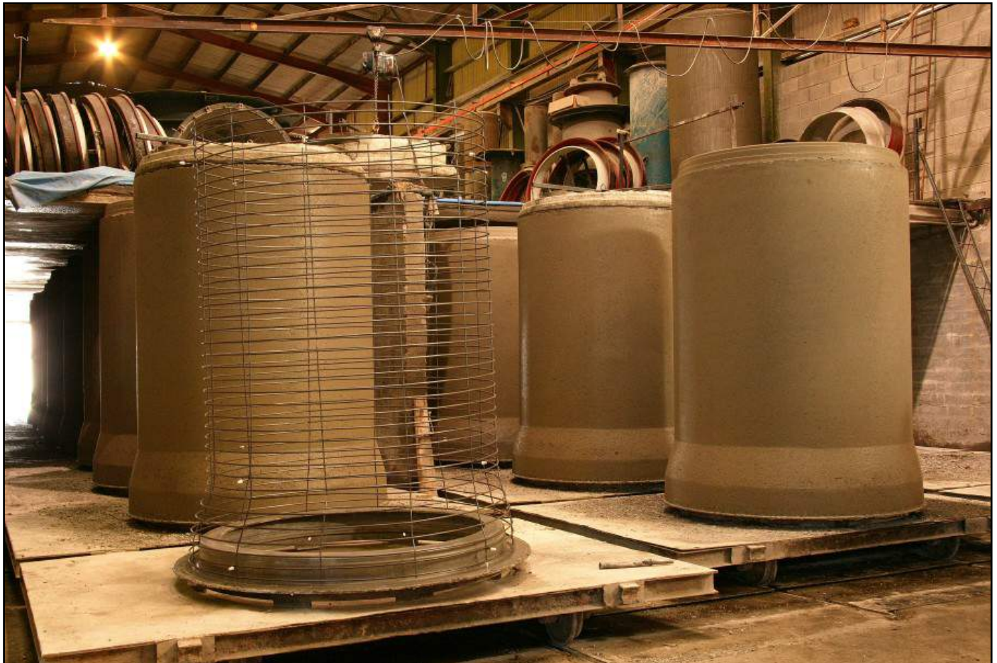
Reinforcement Cage for 1500ø I.S. 6 Pipe
