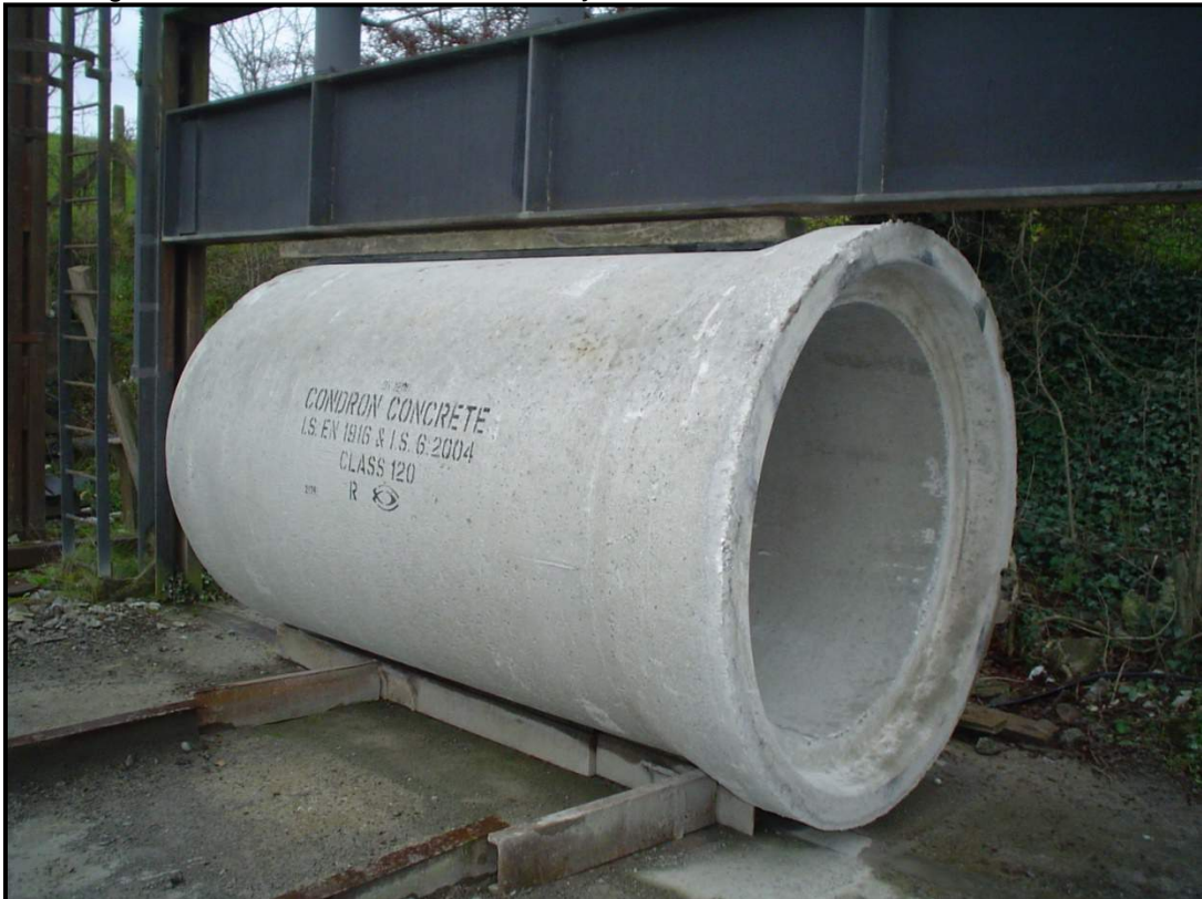
1200mm \varnothing I.S. 6 Pipe undergoing Crush Test
